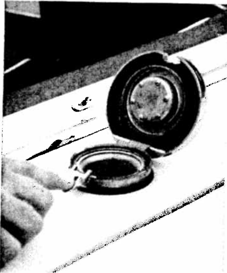
Fuel filler cap is centrally located and has convenient quick-opening mechanism.
